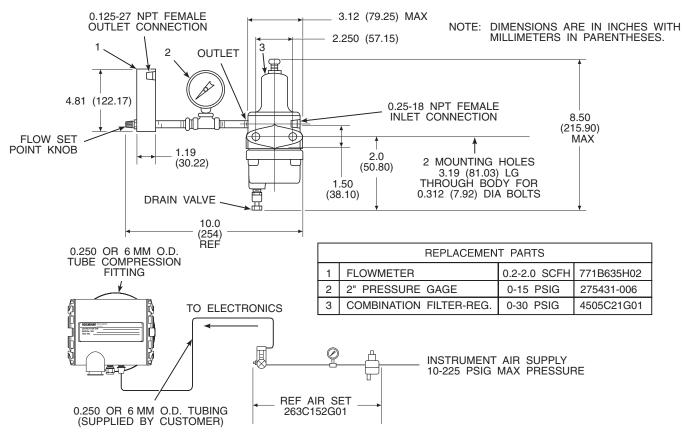
SCHEMATIC HOOKUP FOR REFERENCE AIR SUPPLY ON OXYMITTER DR PROBE HEAD.
